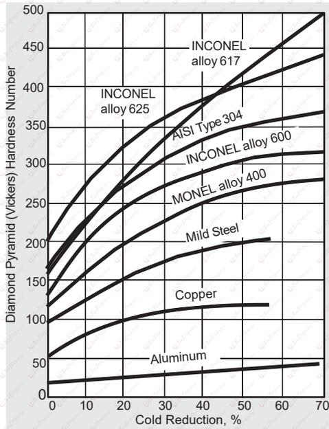
Figure 13. Effect of cold reduction on hardness.
