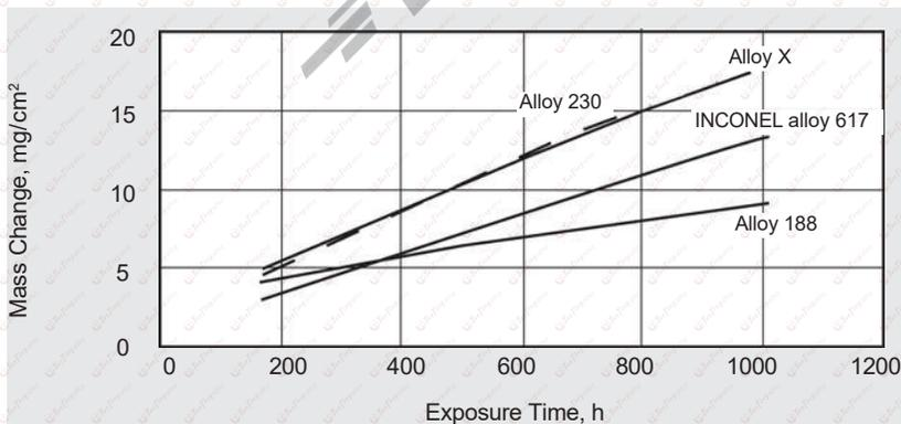
Figure 12. Carburization resistance of heat-resistant alloys at 1832°F (1000°C). Samples were exposed to H<sub>2</sub>-5.5% CO<sub>2</sub>-4.5% CH<sub>4</sub>.
