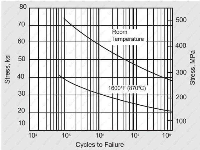
Figure 3. Rotating-beam fatigue strength of solution-annealed INCONEL alloy 617.
